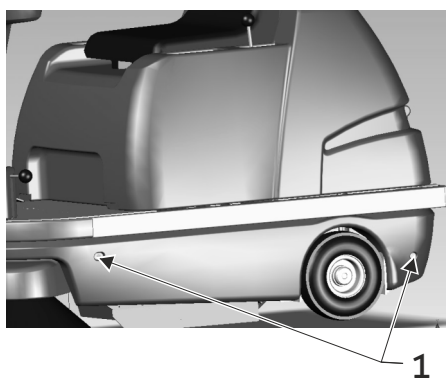
1. Fastening bolts of side trim panel
